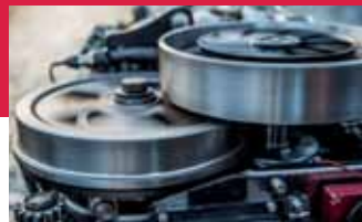
Counter-rotating crankshafts in the powerhead reduce noise and vibration to a minimum.
